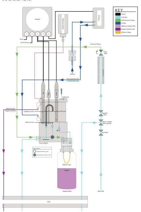
Figure 1: 2109XP Schematic
