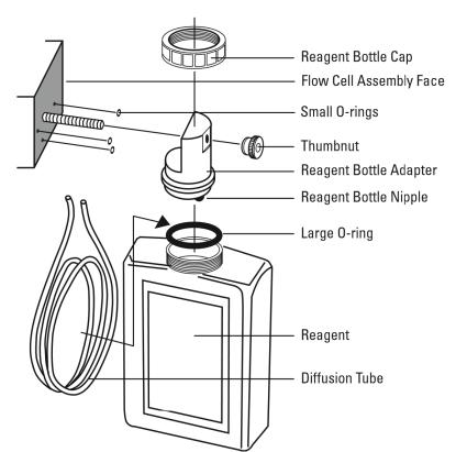
Figure 10: Reagent Bottle Assembly
