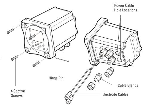
**Figure 7: Electronics Enclosure with Cable Glands**
