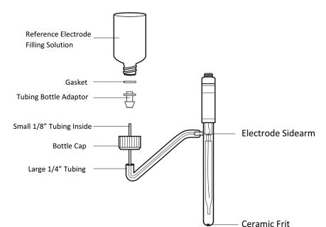
Figure 13: Reference Electrode with Filling Solution
