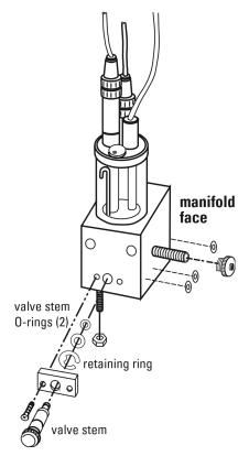
Figure 22: Flow Cell Assembly
