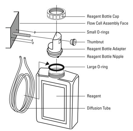
Figure 21: Reagent Bottle Assembly
