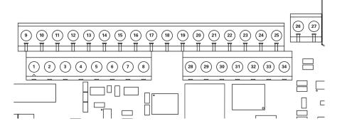
**Figure 9: Terminal Assignments**
