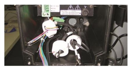
Figure 11: Ferrite Installation
